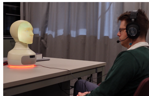
Fig. 5: The setting for the evaluation, showing the red LED lights used in the baseline condition to indicate that the robot is not listening.
